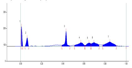
Figure 5. HPTLC finger print of Habb-ul-Neel—Alcohol extract at 254 nm.
