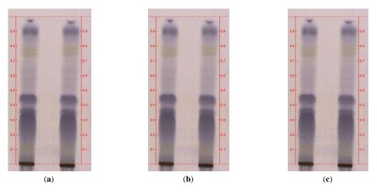
**Figure 4.** Thin layer chromatography (alcohol extract). (a) I N-1, V-S Reagent. (b) I N-2, V-S Reagent. (c) I N-3, V-S Reagent. Solvent System: Toluene:Ethyl acetate (9:1).
