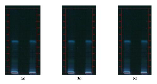
Figure 3. Thin layer chromatography (alcohol extract). (a) I N-1, UV-366 nm. (b) I N-2, UV-366 nm. (c) I N-3, UV-366 nm.
