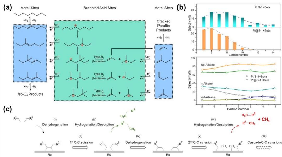
**Figure 9.** The hydrogen-assisted degradation strategies of polyolefins. (a) Mechanism of polyolefins hydrocracking using octane as an example. Reproduced from ref. [140]. Copyright 2021 Elsevier. (b) Distribution of hydrocracking products over Pt@S-1 and Pt/S-1 catalysts. Reproduced from ref. [139]. Copyright 2023 American Chemical Society. (c) Proposed reaction mechanism for the hydrogenolysis on Ru-based catalysts. Reproduced from ref. [141]. Copyright 2021 American Chemical Society.
