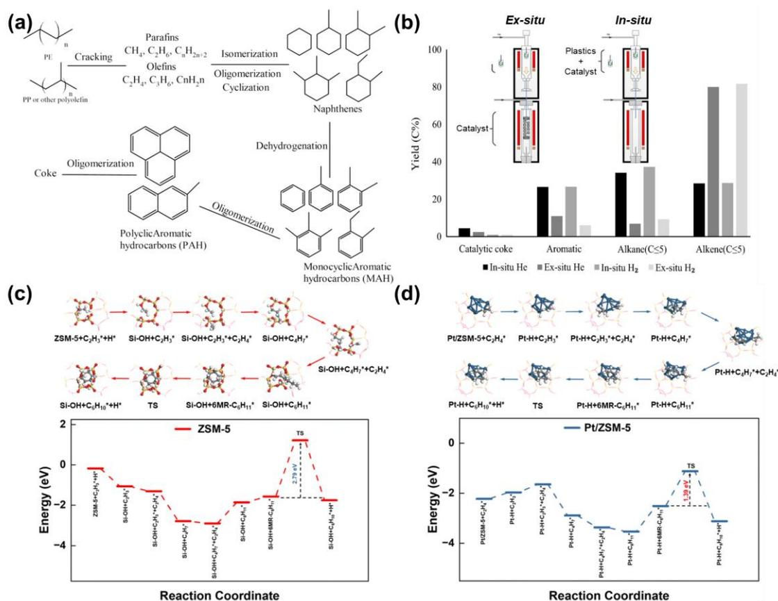
**Figure 8.** Catalytic pyrolysis of polyolefins. (a) Reactions involved in the catalytic pyrolysis process of polyolefins. Reproduced from ref. [121]. Copyright 2024 American Chemical Society. (b) Product distribution during catalytic pyrolysis of PE under in situ and ex situ conditions. Reproduced from ref. [123]. Copyright 2017 Elsevier. (c,d)
