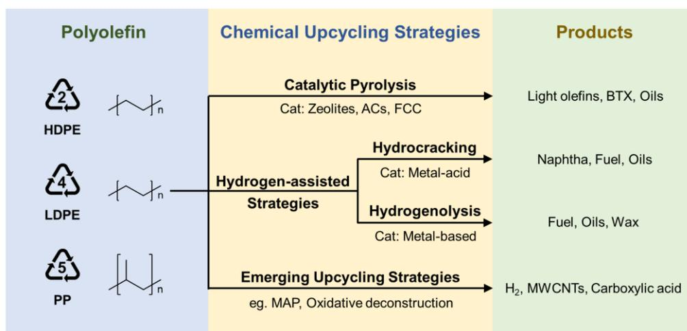
**Figure 7.** Chemical upcycling strategies of polyolefins and corresponding value-added products.
