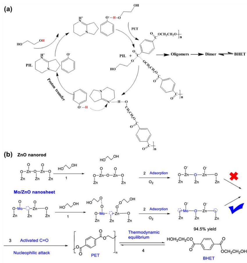
**Figure 6.** Homogeneous and heterogeneous catalytic mechanisms of PET glycolysis. (a) Reaction pathway of PET glycolysis catalyzed by protic ionic liquid. Reproduced from ref. [90]. Copyright 2022 Elsevier. (b) Mechanisms of PET glycolysis catalyzed by heterogeneous ZnO nanorods and Mo/ZnO nanosheets. Reproduced from ref. [96]. Copyright 2022 American Chemical Society.
